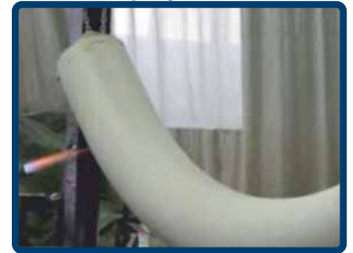
PP Flame Sprayed Bend
