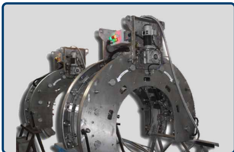
PIPE JOINT MANUAL GRIT-BLASTING EQUIPMENT WITH CONTAINMENT SYSTEM.
